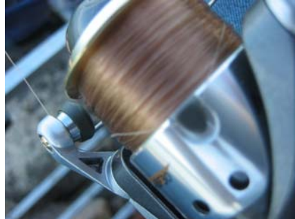
Pic.18: Reel in one turn and trap the line behind the line clip. This fixes the casting distance.
